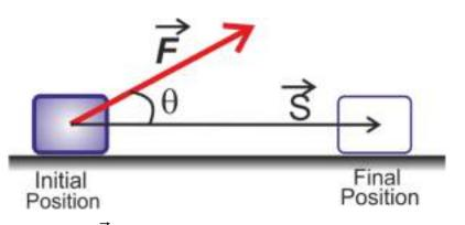
When a force  $\vec{F}$  acts on a body and produces a displacement  $\vec{S}$  then work done by force is given by
